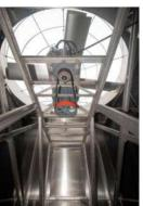
HDGS (Hot Dipped Galvanized Steel), this is a cost effective alternative to casing construction, with good structural strength and adequate corrosion resistance. G235 quality is the highest galvanized grade in the market.
