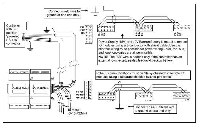
Fig. 4. IO-16-REM-H modules powered by controller connection (RS-485 wiring also shown).
