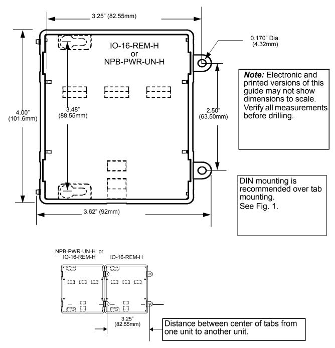
Fig. 14. Tab mounting dimensions.
