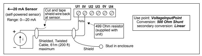
Fig. 10. 4 to 20 mA wiring.
