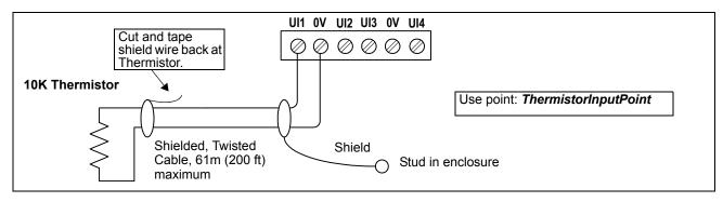
Fig. 8. Thermistor wiring.
