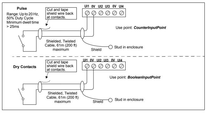
Fig. 11. Binary input wiring.
