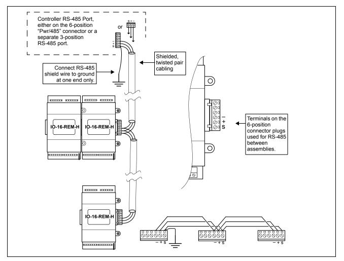
Fig. 7. RS-485 wiring from the controller to one or more IO-16-REM-H modules uses a "daisy-chain" connection.
