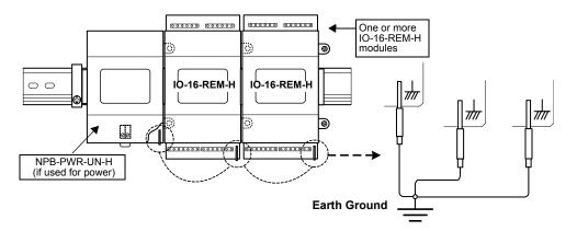
Fig. 3. Earth ground connection required to each IO-16-REM-H module as well as NPB-PWR-UN-H (if using).
