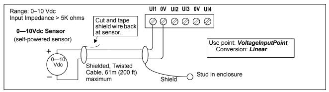
Fig. 9. 0–10 Vdc wiring.
