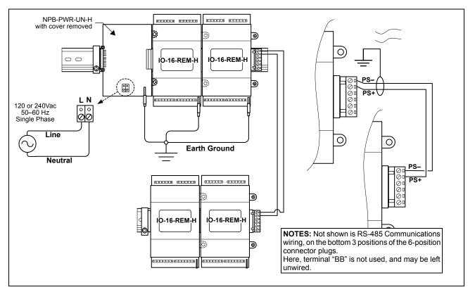
Fig. 5. NPB-PWR-UN-H power supply module used to power IO-16-REM-H modules.
