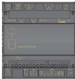
Humidifier control board
